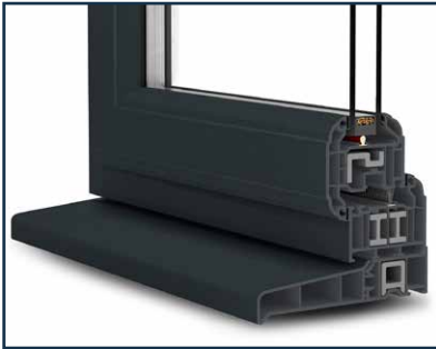
uPVC or aluminium frame windows and doors with thermal breaks and double glazed with 4mm toughened safety glass, argon filled with planitherm coating
